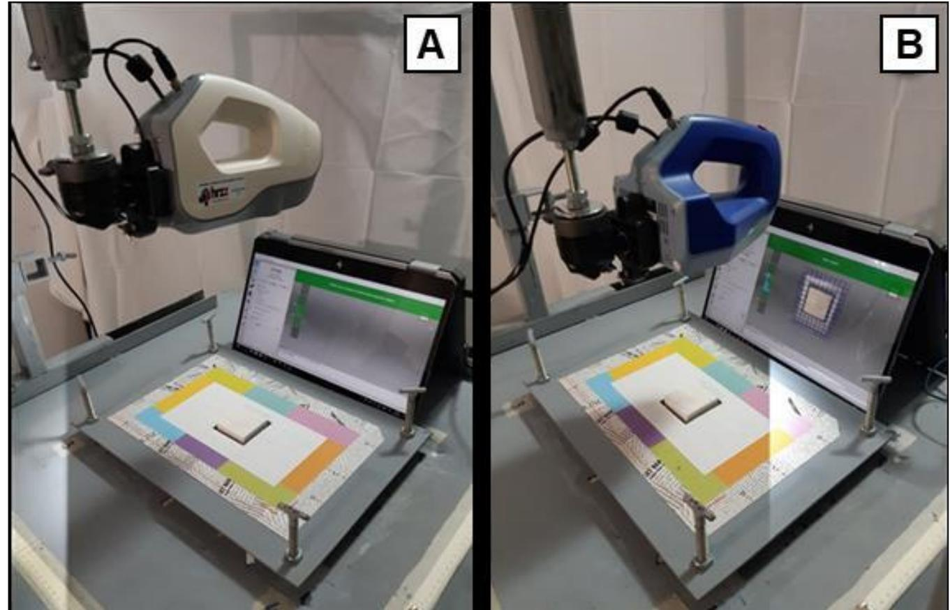
Measurements of the test PL using the *Artec Eva* and *Artec Space Spider* in created **local coordinate system (LCS)**
